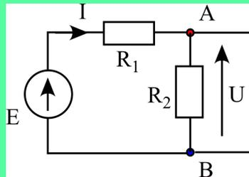
$$U = E \frac{R_2}{R_1 + R_2}$$
