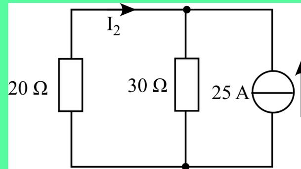
$$\left. \begin{aligned} I_1 &= -\frac{12}{50} \times 5 = -1,2 \text{ A} \\ I_2 &= -\frac{30}{50} \times 25 = -15 \text{ A} \end{aligned} \right\} \Rightarrow I = -16,2 \text{ A}$$
