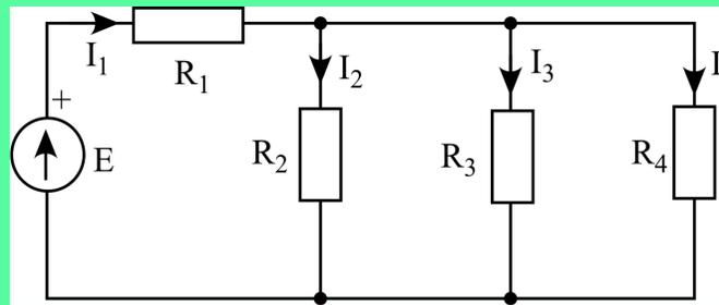
$$\text{On a : } V_{R_2} = V_{R_3} = V_{R_4} = V = E - R_1 I_1 = 100 \text{ V} \Rightarrow R_2 = \frac{V}{I_2} = 100 \Omega$$
