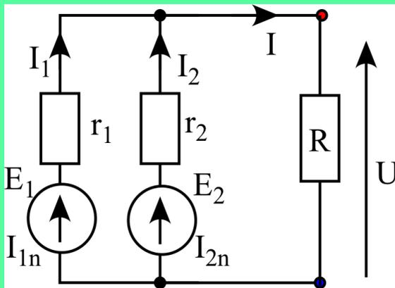
$$E_{TH} = \frac{r_2}{r_1 + r_2} E_1 + \frac{r_1}{r_1 + r_2} E_2 = 49 \text{ V}$$
